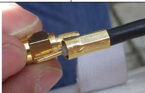
Figure 19; rubber protective sleeve removed.
