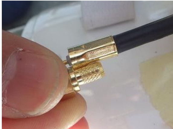
Figure 20 : connector and cable in situation showing the crimped sleeve covering a small part of the connector center.
