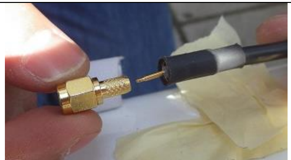
Figure 18: cable with protective sleeve and connector.
