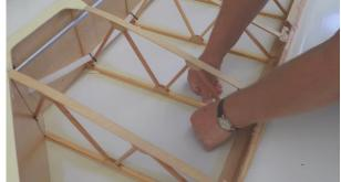
Figure 4: Adherence test of the lower fabric.
