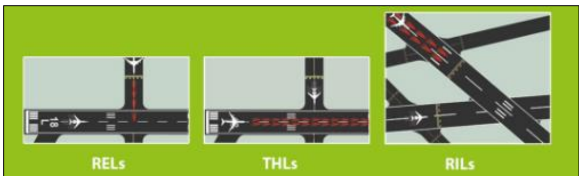
Figure 10 : The different components of Runway Status Lights (picture from Eurocontrol)
