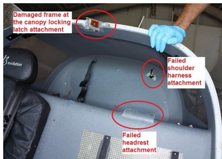
Figure 10: failed shoulder harness and headrest attachment
