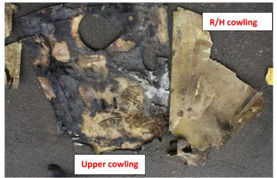
Figure 13: inside view of both the upper and the R/H engine cowlings
