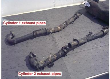
Figure 7: cylinder N°1 and N°2 exhaust pipes
