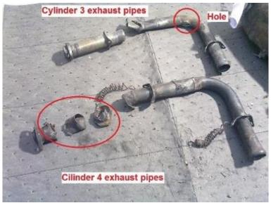
Figure 8: cylinder N°3 and N°4 exhaust pipes
