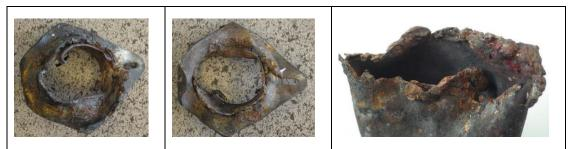
Figure 15: remains of the cylinder N°4 straight exhaust pipe
