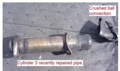
Figure 9: cylinder N°3 recently repaired straight pipe
