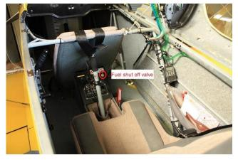
Figure 1: view of the shut off valve control knob
