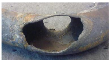
Figure 11: detail of holes in the N°3 exhaust pipe
