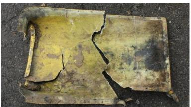
Figure 14: air intake of the water cooler located below the lower engine cowling
