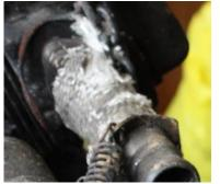
Figure 6: pipe wrapped with a heat resistant tape
