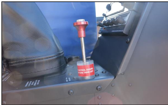
Figure 4: Mixture control (idle cut-off)
