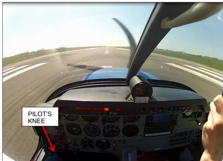
Figure 5: The A/C begins to deviate to the right Time: 2 seconds after touchdown - Airspeed about 61 kt
