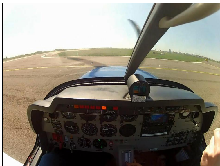
Figure 9: Time 15 seconds after touchdown – Airspeed needle close to the stop
