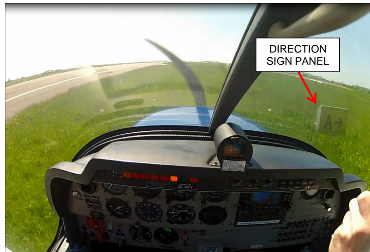
Figure 7: Just before colliding with the direction sign panel Time 9 seconds after touchdown - Airspeed 45 kt (Edge of the white arc)
