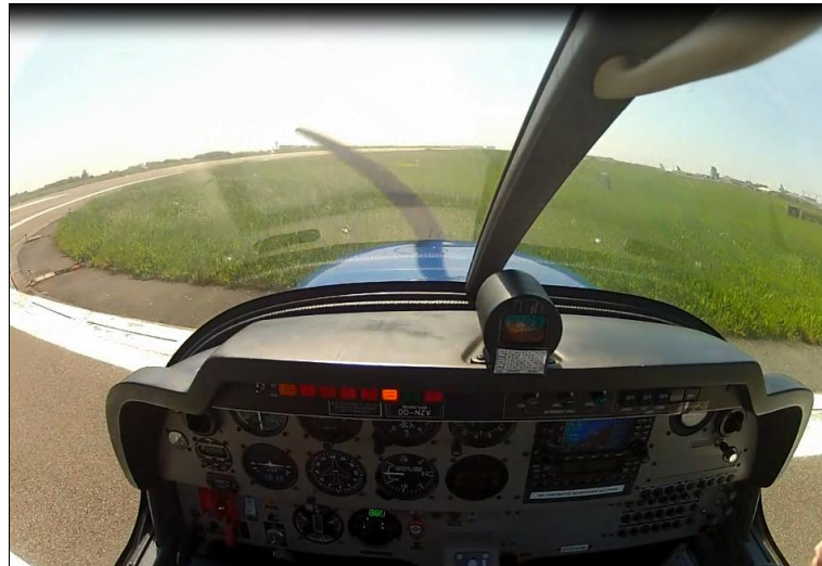
Figure 10: Time 19 seconds after touchdown, just before stopping Airspeed needle on the stop
