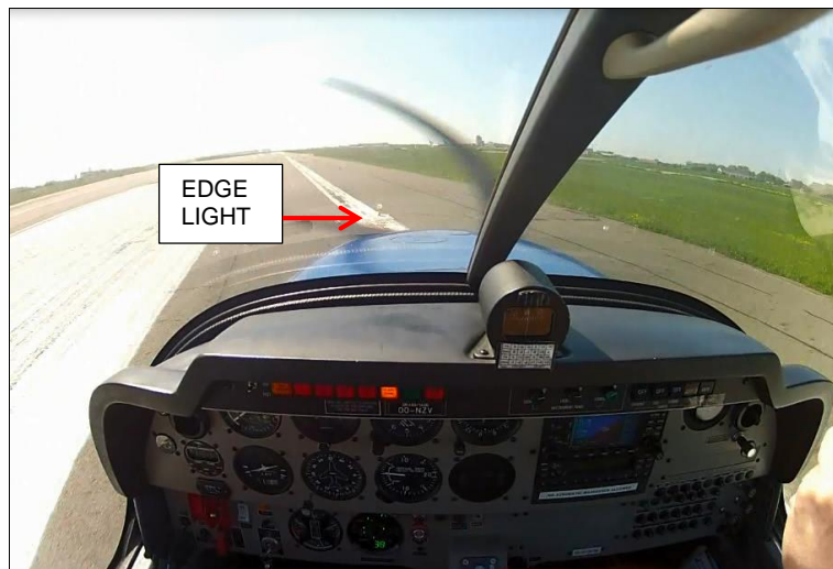
Figure 6: Just before hitting the edge light with the left wheel fairing Time 6 seconds after touchdown – Airspeed 52 kt
