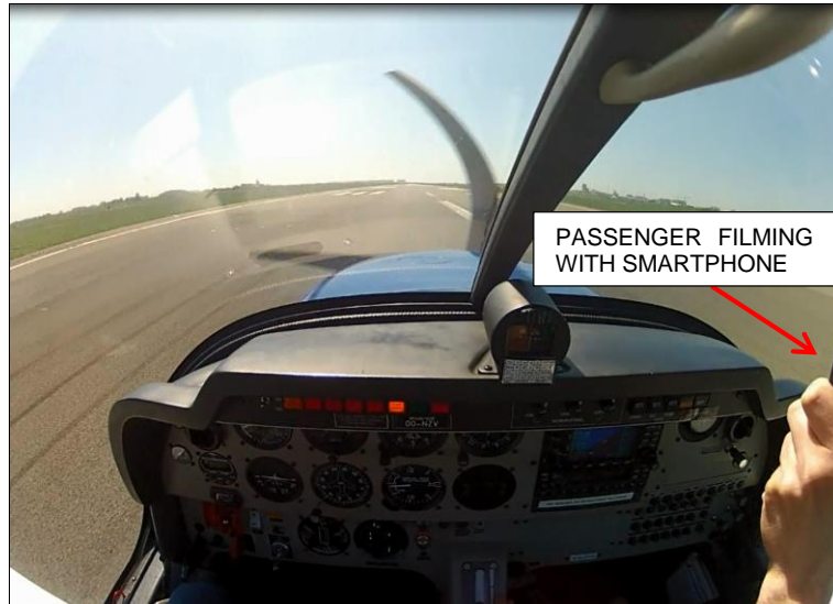
Figure 4: Touchdown – reference time: 0 – Airspeed about 62 kt
