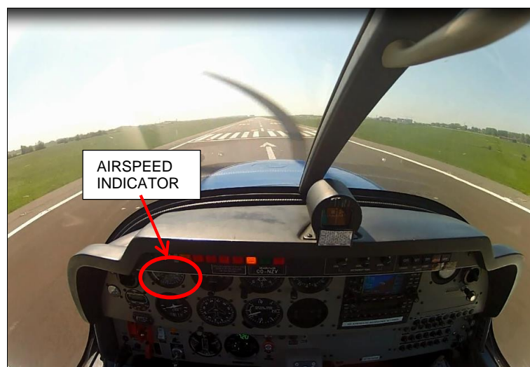
Figure 3: Aeroplane in flight – The airspeed needle is not yet visible
