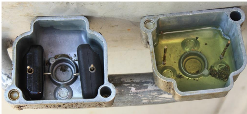
Figure 3: carburettors' bowl showing the presence of contaminant.
