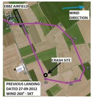
The hereby enclosed picture shows a turn made when a 5KTS wind was coming from 260°.
