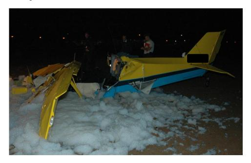
The BRS parachute had not been activated and its control cable had been deactivated by the rescue services for safety.
