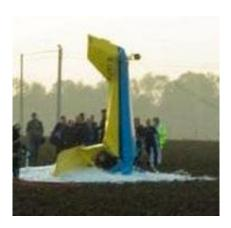
The airplane collided with the ground vertically and remained in vertical position after the crash until the rescue services cut the wing rear attachment in order to gain access to the victims.
