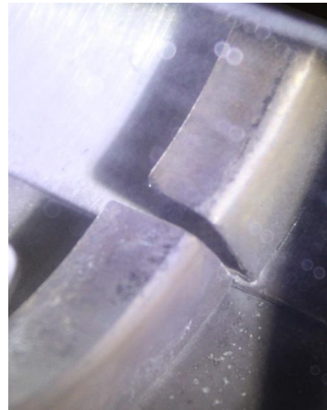
Figure 11: View of misaligned central ribs located between carburettor heat and cabin heat chambers
