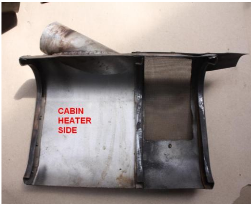
Figure 9: View of black deposits located inside the shroud, only on carburettor heat side
