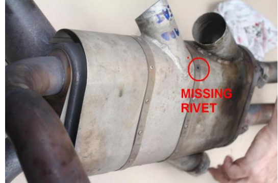
Figure 8: missing rivet on carburettor heater shroud
