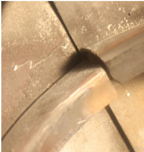
Figure 11: View of misaligned central ribs located between carburettor heat and cabin heat chambers
