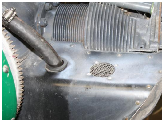
Figure 12: View of the cabin heat air intake screen featuring square openings significantly larger than the wire mesh of the carburettor heat shroud.
