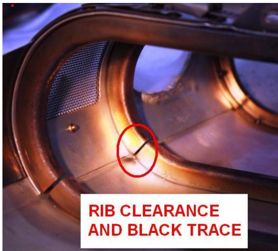
Figure 18: Newly installed shroud
