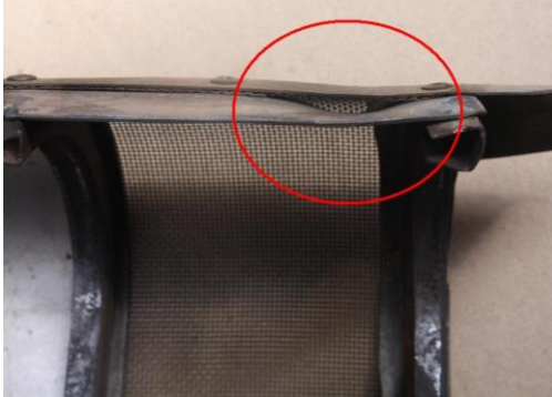
Figure 7: example of mesh wire support damage
