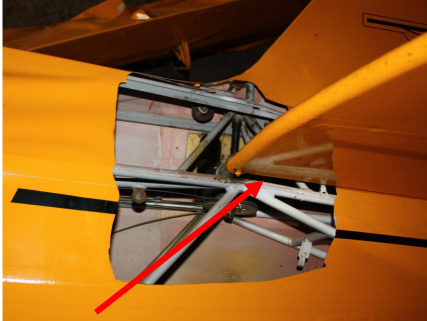
Figure 13: End position of trim jack screw
