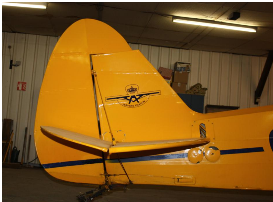
Figure 5: Example of a stabilizer in full nose up position. Notice the up-position of the elevator
