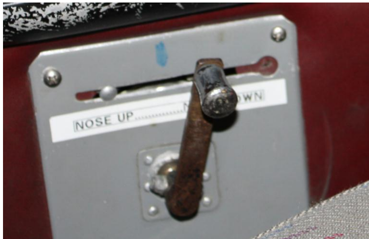
Figure 6: Stabilizer trim control of another PA-18
