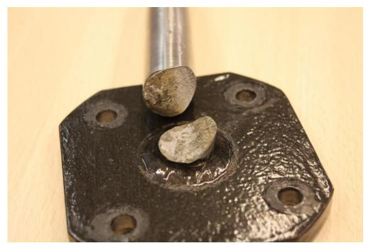
The axle of the nose landing gear fork was found broken at the junction of the square base.
