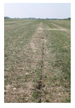
The airplane nose landing gear leg left a 5 meter long groove in the ground.
