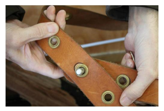
One of the two ventral straps was provided with a fixed pin while the other ventral strap was pierced with a few holes to allow the pilot to adjust the length of the straps.
