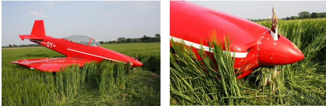
Figure 1: General view of the A/C and damages to the propeller.
