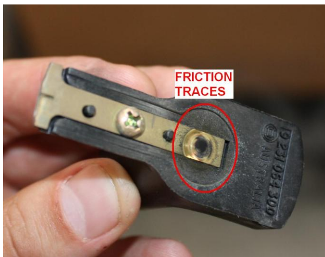
Figure 5: Friction traces on a practically new rotor
