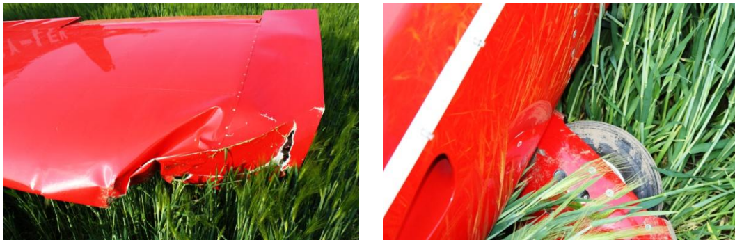
Figure 2: L/H wing leading edge and view of the nose wheel under the engine cowling.
