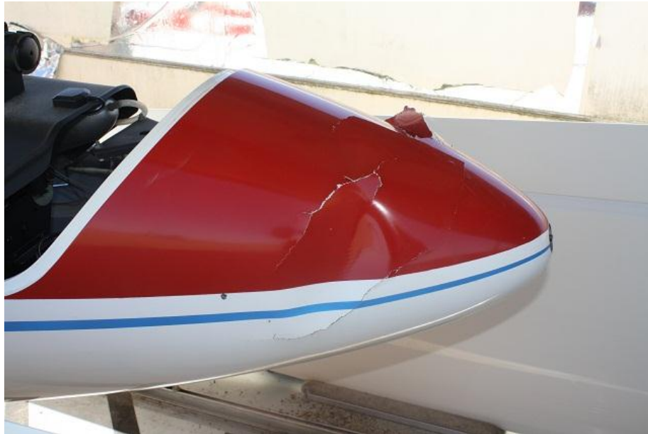
Fig. 1 Damage to the nose of the sailplane
