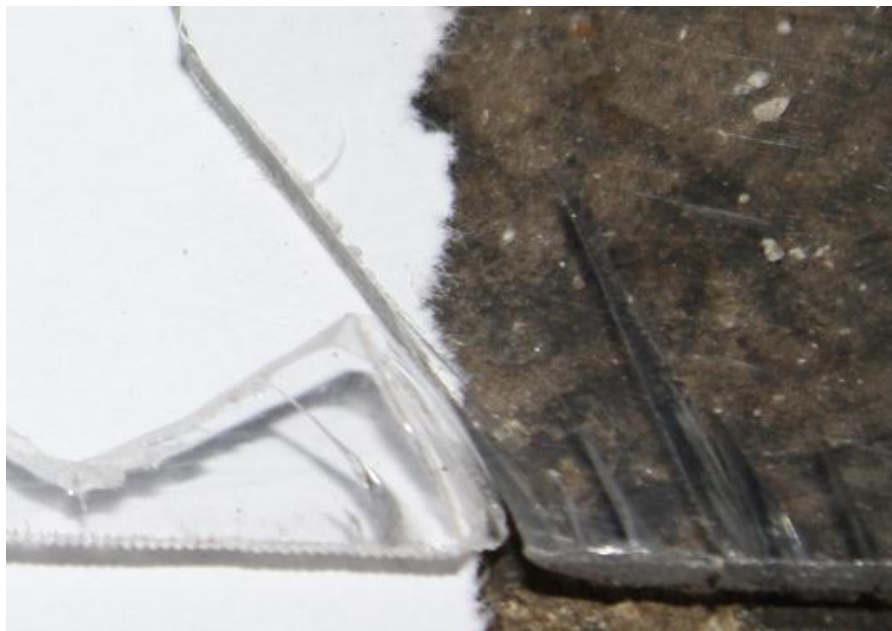
Fig 10 cracks in the windscreen
