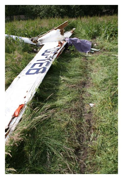
The deformation of the wing show a near-frontal impact with the ground.
