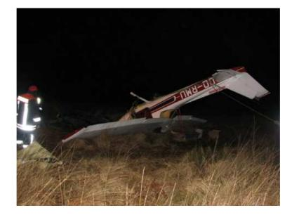
The ground is a peat bog, quite soft and marshy, and the aircraft decelerated rapidly. The Nose Landing gear hit a trunk and the aircraft overturned.
