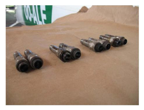
These conditions are compatible with the icing conditions and the report of witnesses showing "black smoke" through the exhaust.
