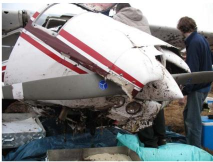
The engine cowls are damaged.
