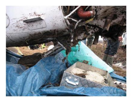
The RH main LG wheel axle is severed.
