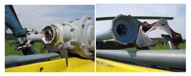
The intermediate rupture of the shaft is due to a contact between the shaft and one of the main rotor blade; yellow and blue paint were found on the "yellow" blade.
