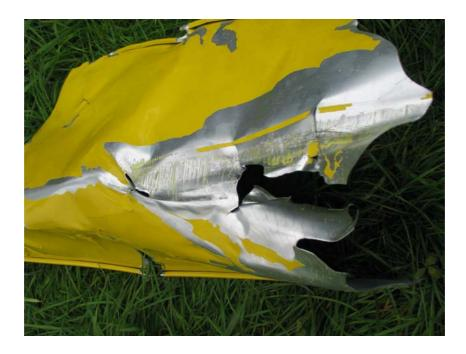
The last rupture shows the characteristics of a bending rupture; the shaft is bent for over  $90^{\circ}$
