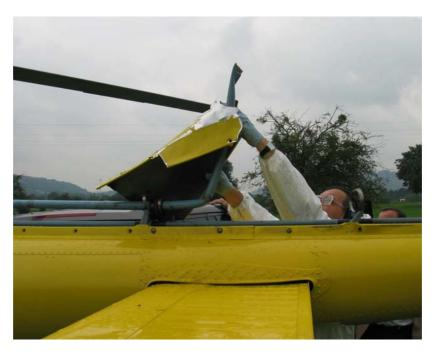
The inspection of the rupture faces shows there were due to high loads. There was no obvious indication of corrosion or prior cracks.
