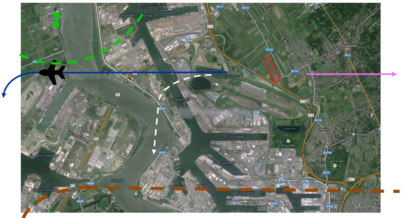
When leaving Hoevenen: Wishing to remain outside of controlled airspace, **on a westerly heading**, turn south only when the **nuclear power plant (landmark: cooling towers) of Doel** is beyond your 3 o'clock position. **VOR Radial 020 of NIK (Nicky) VOR** can be used for guidance, to remain clear of the Antwerp CTR. NOTE: The nuclear power plant of Doel is a MR-area (Military Restricted). Overflight by civil aircraft is not stimulated, but not forbidden, nor fined.
